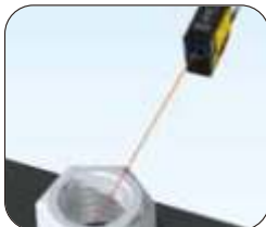
Checking for the presence of threads
