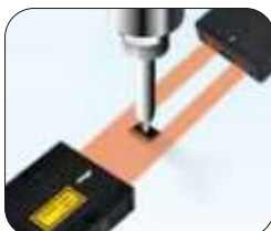
Locating a small IC chip held by a vacuum pickup
