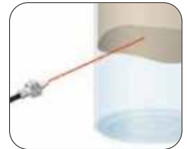
Level check of water
