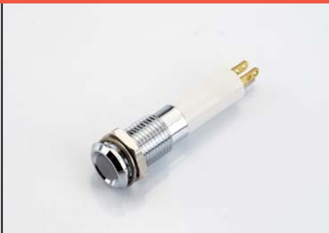
Piloto, reflector plano, LED 5mm, 24VDC, montaje 8mm, tricolor
